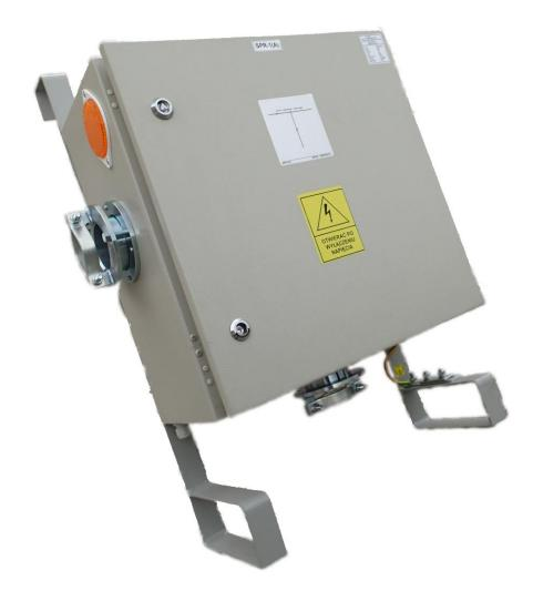
Switchgear type SPR-1A is an electrical devices designed for use in the underground mining faces in non-explosive hazard conditions and on the ground in environment 2. Switchgear type SPR-1A is designed for connecting and branching-off mine 3-phase grid circuits with insulated star point of the transformer (IT system) for the grid rated voltage of 500V.
